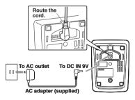
4) Charge the handset battery pack for at least 15-20 hours before using your new handset for the first time.
